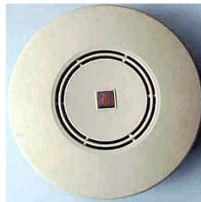
A smoke alarm
